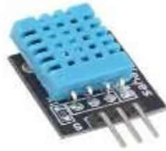
Fig. 3 DHT11 Temperature and Humidity sensor
