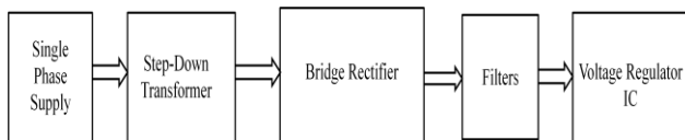
Fig 2 Power Supply Block
