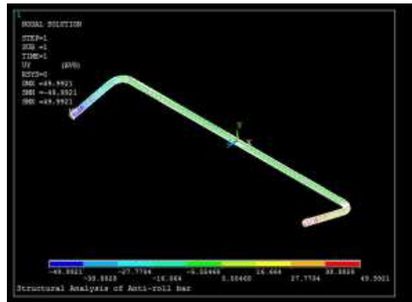
Fig.10. Displacement of Anti-roll bar in Y-direction
