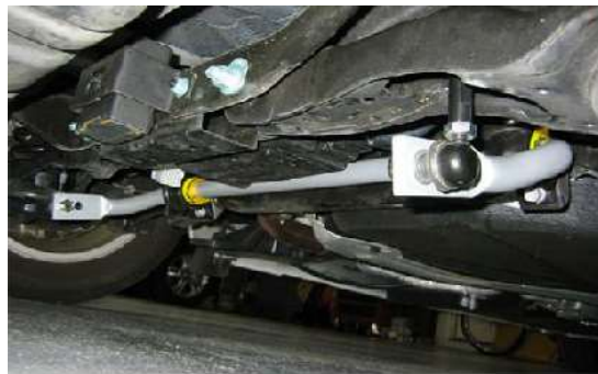
Fig.1. Fitment picture of Anti-roll bar on vehicle [3]
