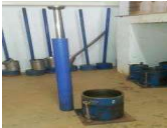
Fig.3 modified proctor apparatus
