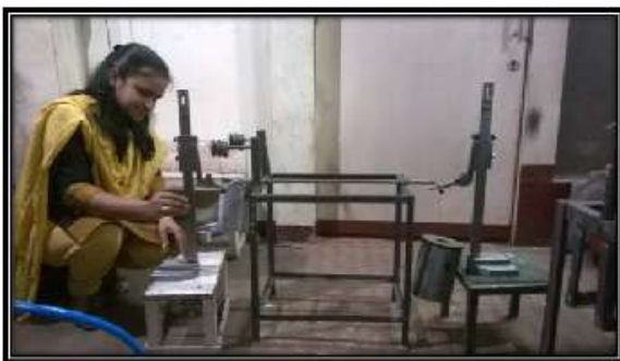
Figure3. Experimental setup of anti-roll bar for finding deflection
