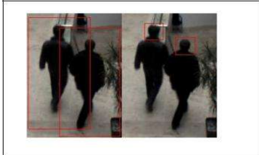
Figure 1: Example results after applying the HOG detector for pedestrians (left) and heads (right)
