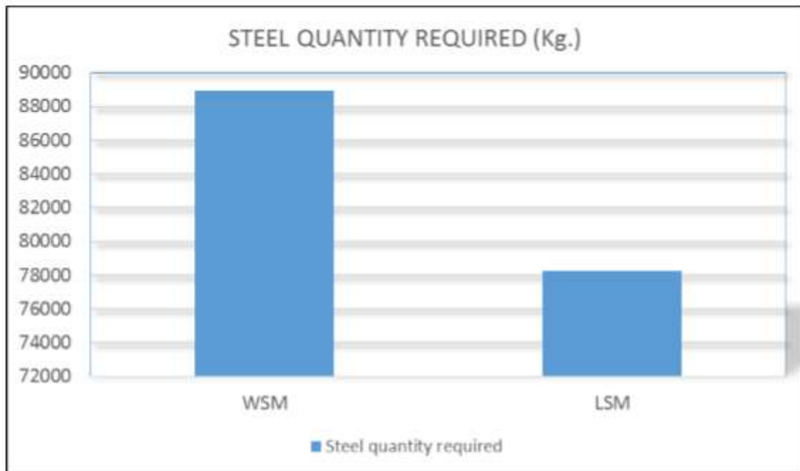
Figure No.5 Comparison Required Steel Quantity
