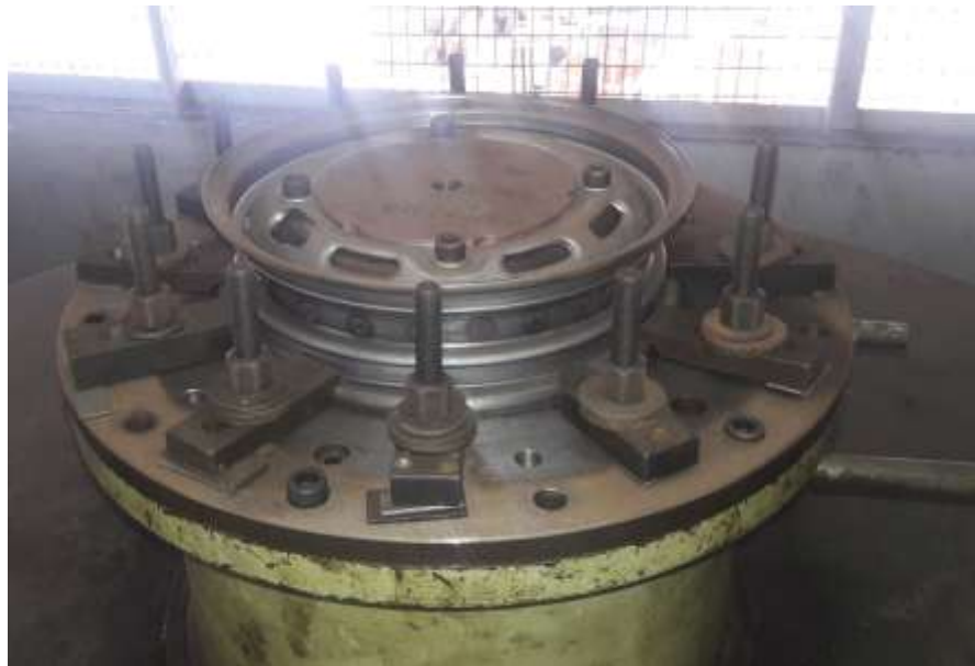
Photograph of Dynamic Cornering Fatigue Test Setup
