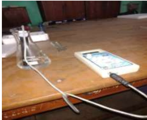
Fig 5. Digital DO meter used for testing DO in wastewater
