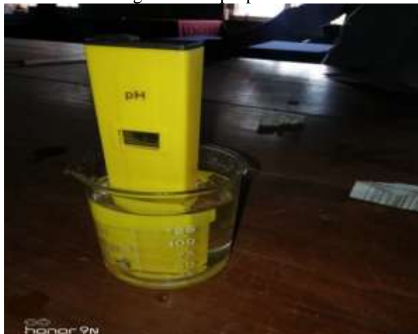
Fig 3. Digital pH meter used for testing pH of wastewater
