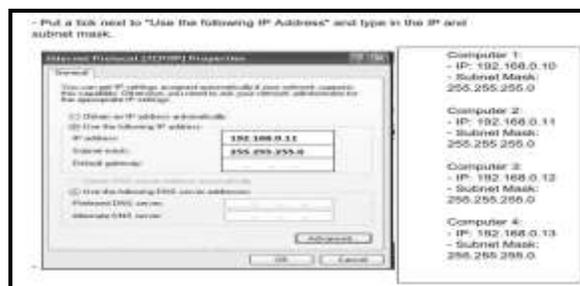
Fig.: Internet Protocol (TCP/IP) Properties - setting IP address
