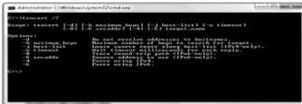
Fig.: Output screen of command C:\>tracert /? Help
