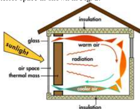
Fig-2 Trombe wall with air circulation open during day and closed in night.
