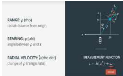
Fig 6: Measurement function of the RADAR sensor
