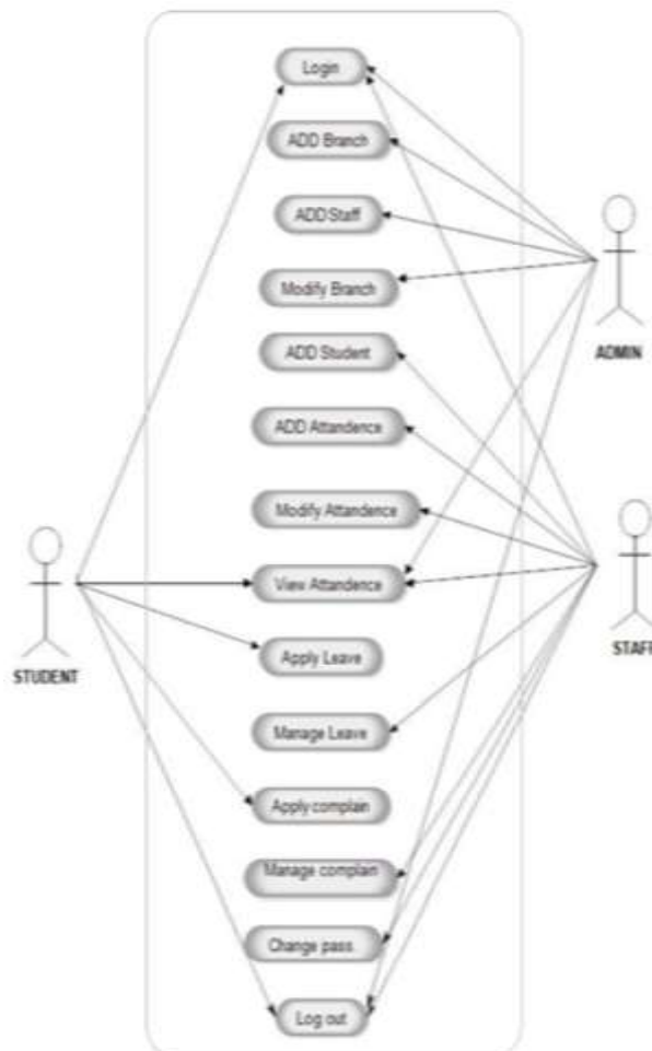
Figure 1 The diagram shows different users and their different access for interaction within the system with the help of entities. Unlike students and faculty, Admin can have all use case entities.
