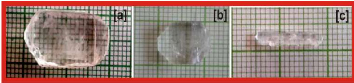
Fig -1: Crystal of (a) KDP, (b) CA:KDP and (c) GA:KDP
