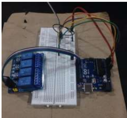
Fig-3: Electrical Components - 4 linear flex sensors relay circuit, Arduino, Jumper cables, breadboard
