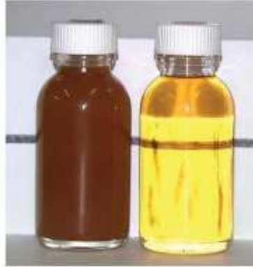
Fig 2: Transformer Oil Before and After
