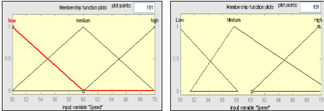
Figure 8: Initial and final membership function for cutting speed for MRR
