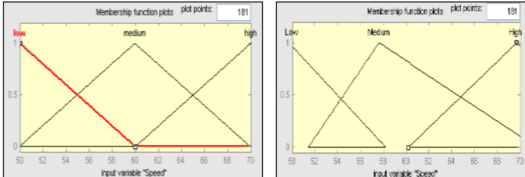
Figure 5 Initial and final membership function for cutting speed for Ra
