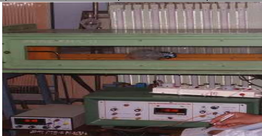
Figure 6, Testing of Tata Indica Car on Wind Tunnel
