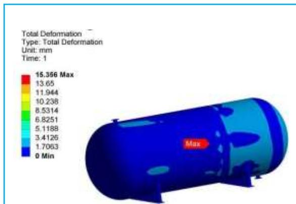
Figure 20:-Total Deformation results
