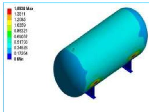
Figure 7:-Maximum Deformation=1.5538 mm
