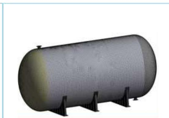
Figure 23:-Mesh Modified Model
