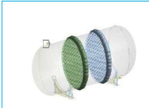
Figure 18:-Pressure Vessel with 2 Saddle Supports
