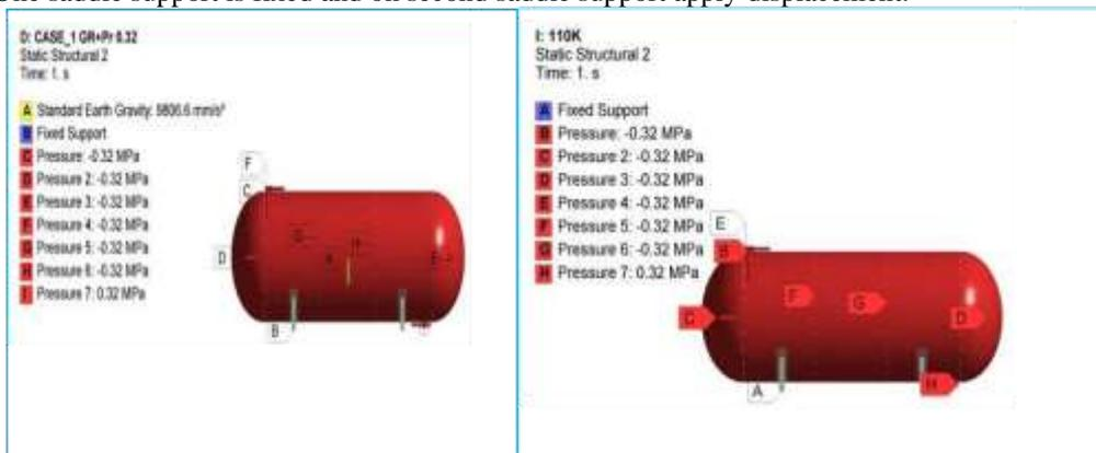
Figure 10:-Boundary conditions for Case 1 Figure11:-Boundary Conditions of fixed support Applying Internal Pressure of 0.32 MPa on all bodies of Pressure Vessel.
