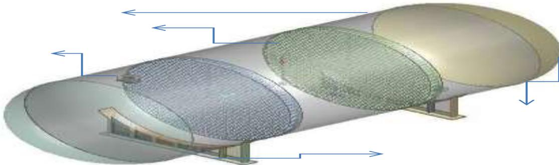
Figure 2. Cad model of horizontal heat exchanger
