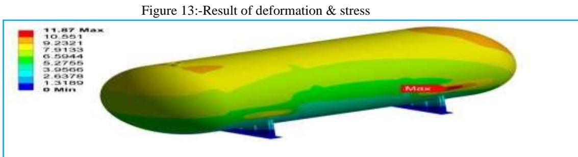
Figure 13:-Result of deformation & stress
