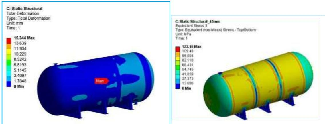
Figure 24:-Maximum Deformation=15.344 mm    Figure 25:-Maximum Stress=123.18 MPa
