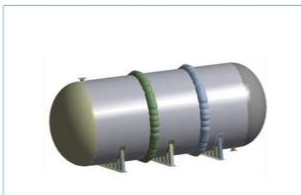
Figure 22:-Pressure Vessel with 3 Saddle Supports
