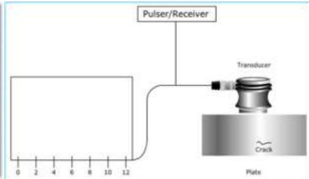
Figure 28:-Systematic diagram of UT Testing
