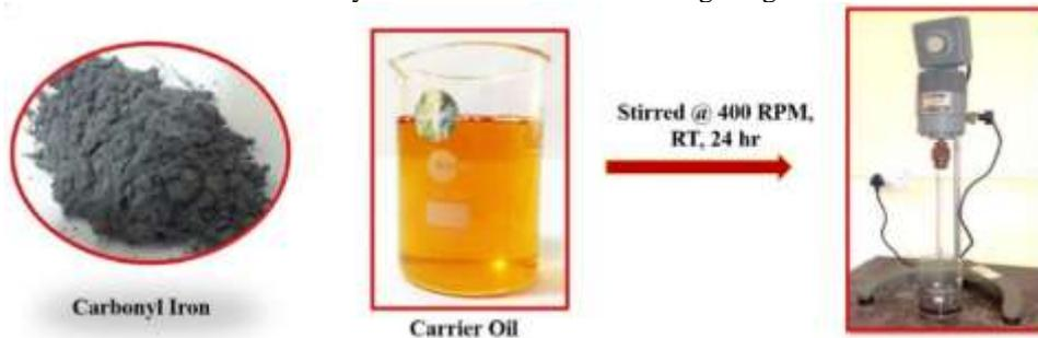
Fig. 1 Scheme of preparing of MR fluid
