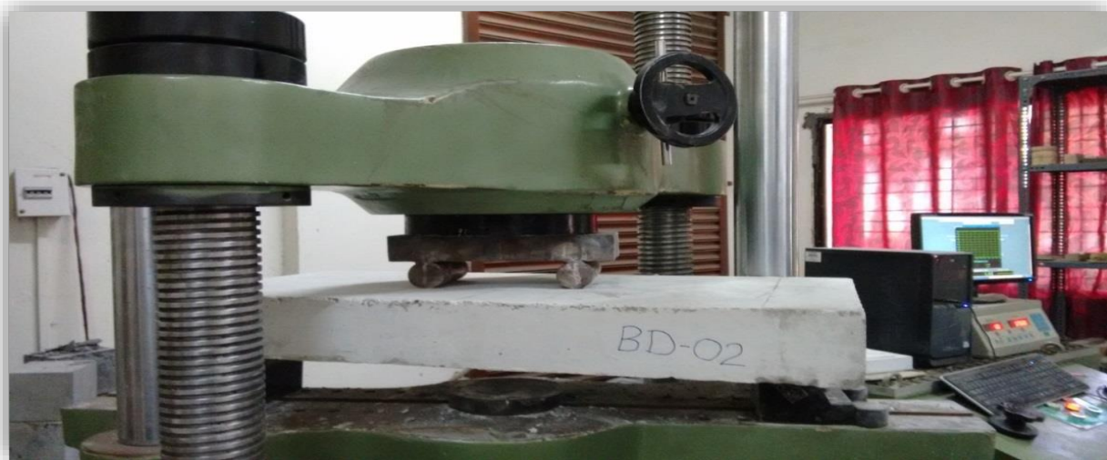
Fig.7 100 mm Thick Panel Under Two Point Loading System (Flexural test)
