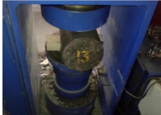
Fig -3 Set up for split tensile test
