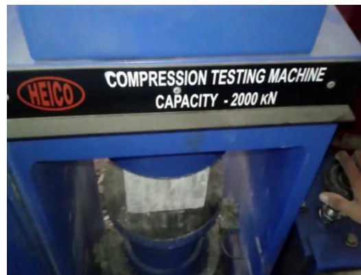
Fig -2 Set up for Compression test
