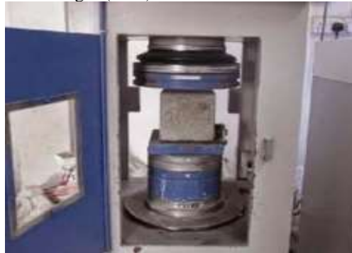
Fig -1: Compression Testing Machine for Cubes
