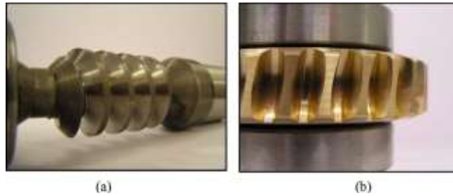
Fig-4. (a) The new worm screw gear (b) the new crown gear.
