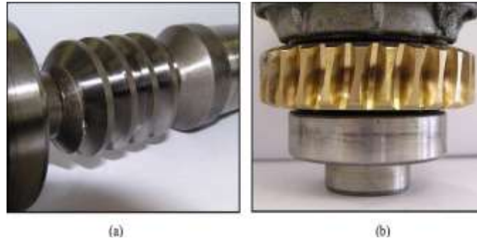
Fig- 9 (a) Worn surface of the worm screw gear after test Fifth; (b) worn surface of the crown gear after test fifth
