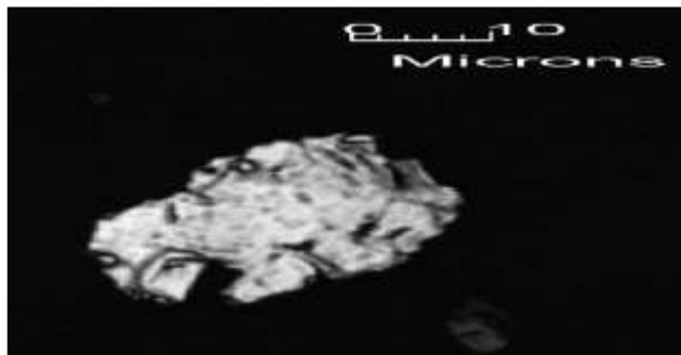
Fig- 8 Representative laminar particle from test five.
