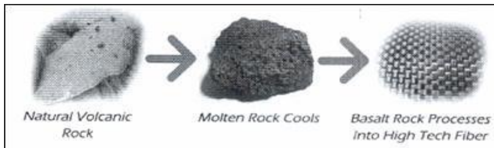
Figure 4: Formation of basalt fibre
