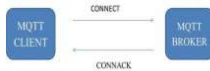
Fig 3 MQTT Client and broker link
