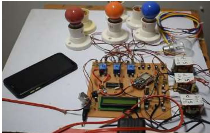
Fig -4 Working model of IoT based Transmission line Monitoring System.
