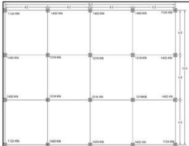
Plan & column reaction of G+5 building
