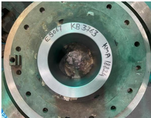
Fig-3 Prepared token (valve sleeve) for cladding
