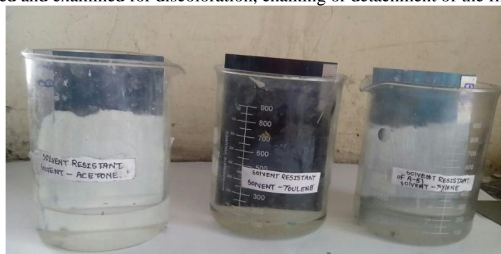
Photo 4 – Solvent Resistant Test
