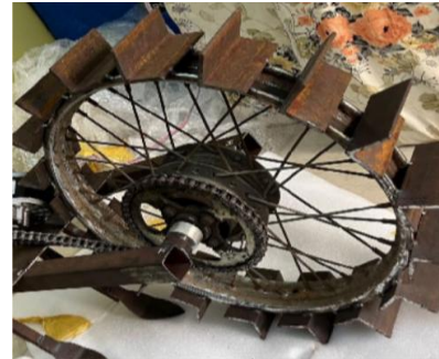
Fig 5.3 – Tilling blades welded on wheels
