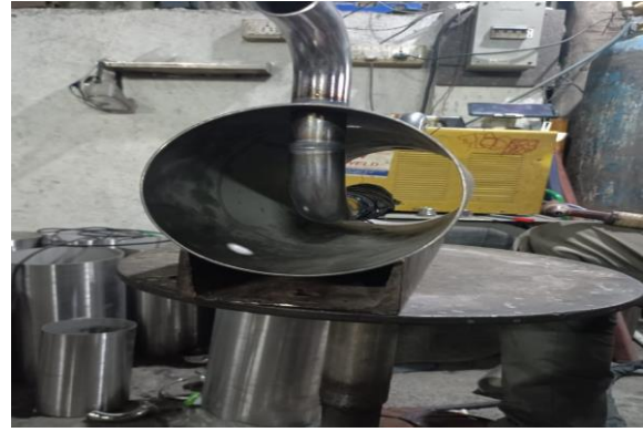
Fig 4.4 - Lime and Water Chamber
