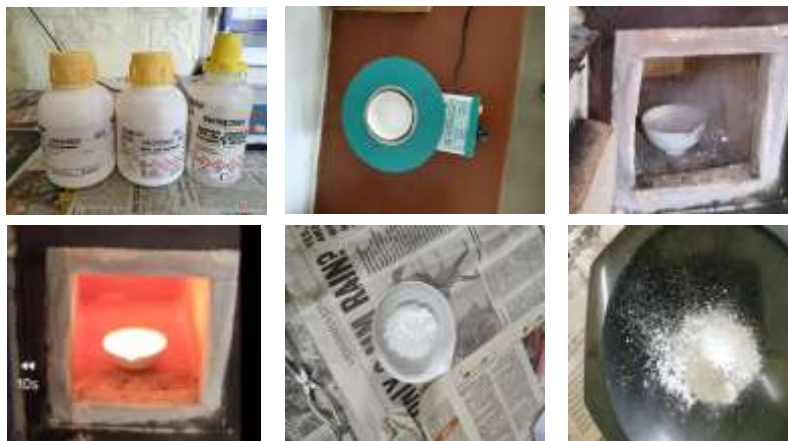
Fig. 1 Stepwise synthesis of phosphor by solution combustion technique.
