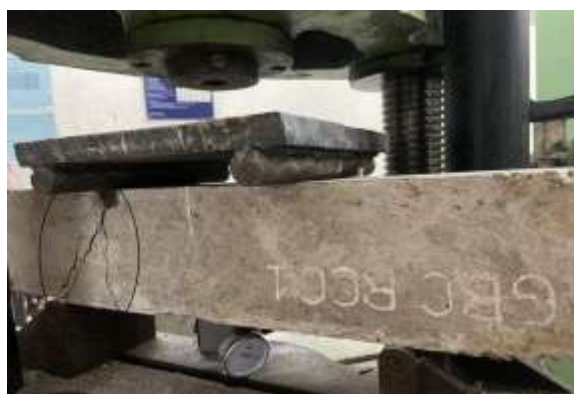
Fig. 10 Flexural Tension Failure in Grooved Bamboo Coating Reinforced Cement Concrete Beam
