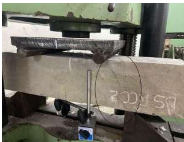
Fig. 11 Flexural Tension Failure in Bamboo Steel Reinforced Cement Concrete
