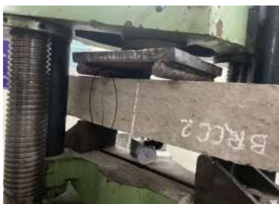
Fig. 8 Flexural Tension Failure in Reinforced Cement Concrete Beam
