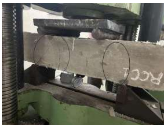
Fig. 8 Flexural Tension Failure in Reinforced Cement Concrete Beam
