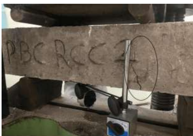
Fig. 10 Flexural Tension Failure in Bamboo Coating Reinforced Cement Concrete Beam
