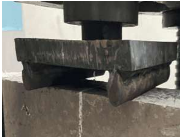
Fig. 6 Beam Testing Setup
