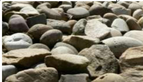
Figure 2: Crushed coarse stone aggregates of nominal size 20 mm.
