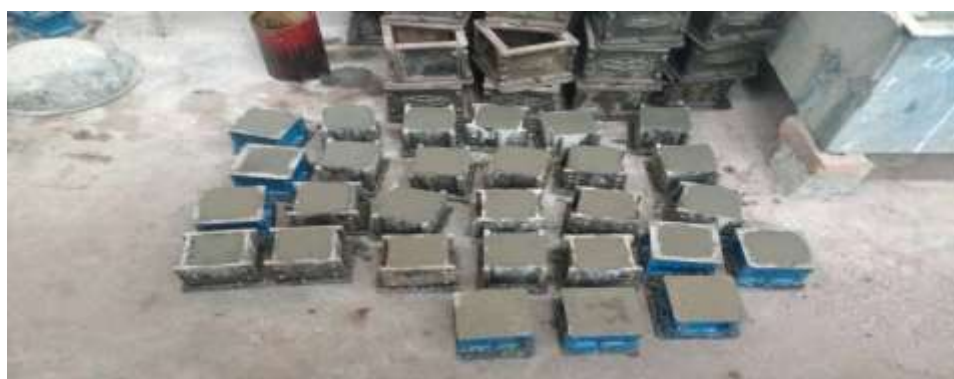
Figure 5: Casted cube specimens
