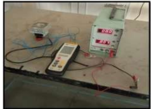
Fig 4 :- Experiment of plate fin Heat sink by Natural convection
