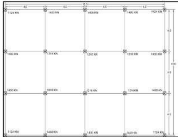
Plan & column reaction of G+5 building
