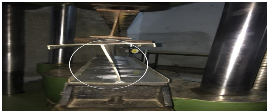
Fig 4 Lateral torsional buckling in web of cold formed I section without intermediate stiffener
