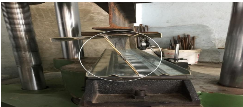
Fig 5 Lateral torsional buckling in web of cold formed I section with intermediate flange stiffener
