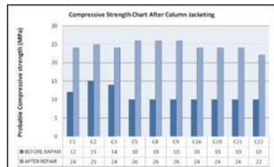
Graph 2: Comparison of Compressive Strength with Rebound
