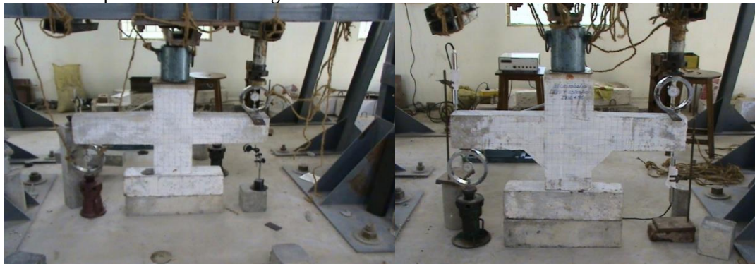
Fig.7&8: Test Setup for specimens CS & HS 1(Forward Loading Position)
