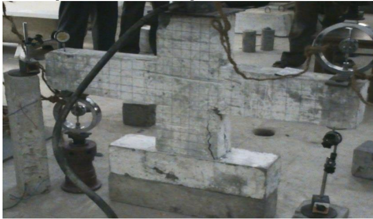
Fig 17: Failures of control specimen (CS) and haunch specimen ( HS 1)
