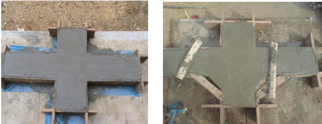
Fig 6: Casting stage of test specimens CS & HS 1
