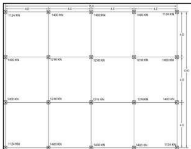
Fig -1: Plan & Column Reaction of G+5 Building
