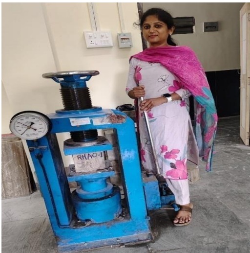
Figure 1 Rice Husk Ash Cube Testing
