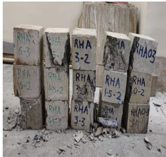
Figure 2 Rice Husk Ash Cube after Test
