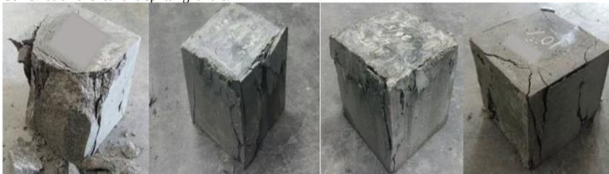
Figure No 2. Modes of failure of the specimen
