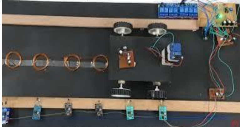
Fig-2: Dynamic wireless EV charging road embedded coil.
