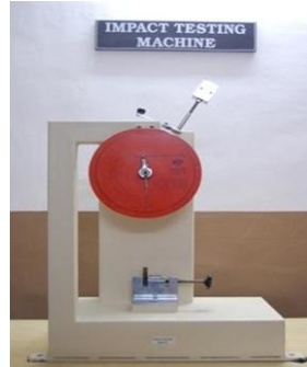
Fig -2: Analog Izod/ Charpy impact tester [4]
