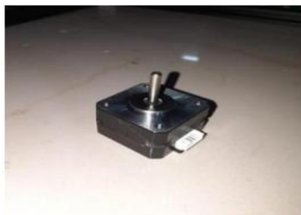
Figure 4(a)- Stepper Motor
