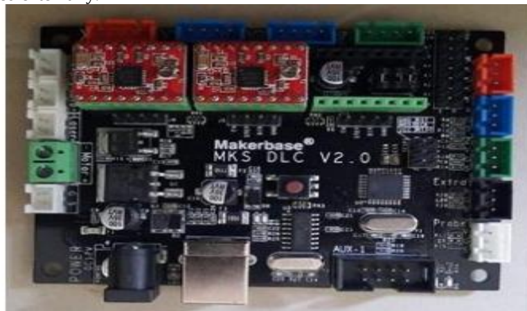
Figure 2 - MakerBase Control Board
