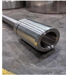
Fig 3. Surfaces to be Hardened
