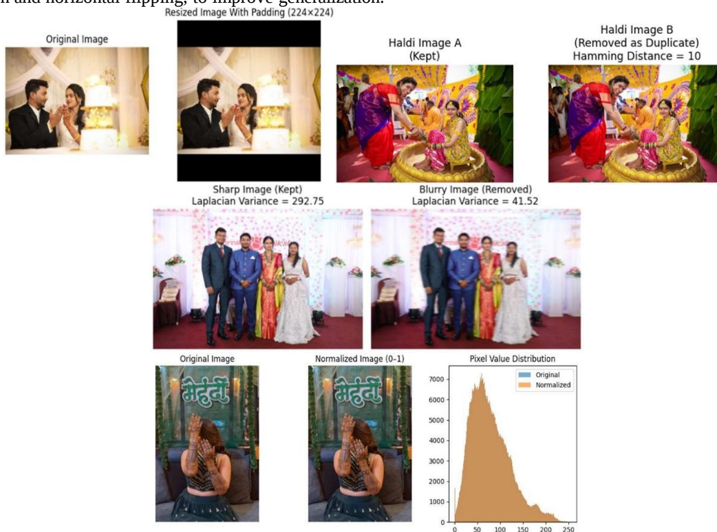
Fig -2: Sample results of image preprocessing showing resizing with padding, normalization, and removal of duplicate and blurred images.
