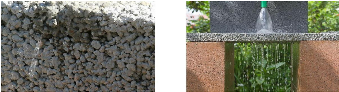
Fig 1: Porous Concrete (Permeable Paving) [2]
