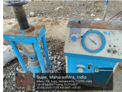
Fig No. 3.7- Compressive Strength Test
