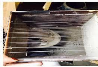
Fig No. 3.6 – Fiber Arrangement in Concrete Mould
